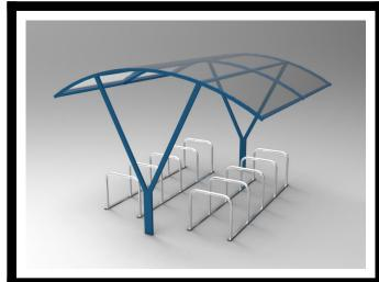
Designed to double the number of cycles you can fit in a relatively small space, with 2 rows of bike parking. This Cycle Shelter is available in a galvanised or powder coated RAL code colour finish with galvanised cycle stands. Anti-climb roof and end frames with 3mm polycarbonate panels on the roof.
