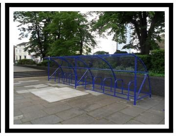
Our best selling cycle shelter, comes with the best all-round features to suit any environment. Mild steel shelter with boltdown fixing. Shelter available in a galvanised or polyester powder coated RAL code colour finish. Anti-vandal clear 4mm polycarbonate roof, with optional polycarbonate sides and swing or sliding gates. Comes with optional cycle parking, galvanised bike stands.
